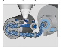
In its standard configuration a powder mixer has a compact design consisting of a tube frame on mounting feet or wheels, a funnel, table, manual disc valves and connecting pipes. The table top at an ergonomic level provides for easy manual feeding.
